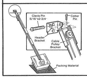
PROCEDURE: Position opener chassis on garage floor below door and header brackets. Use packing material base to protect cover. NOTE: To enable Tee rail to clear sectional door springs, it may be necessary to lift the chassis onto a temporary support.
